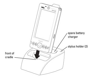
**4** Align the connector on the bottom of the device with the connector on the cradle, and, keeping the front of the device flush with the front of the cradle, lower the device onto the cradle.
